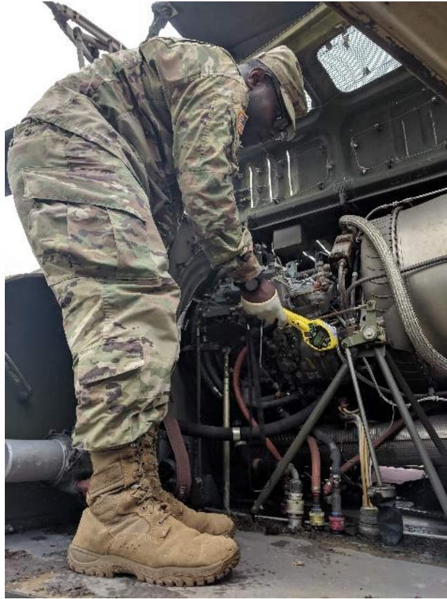
Figure 2. Surveying a Helicopter Engine Made of Magnesium-Thorium Alloy
